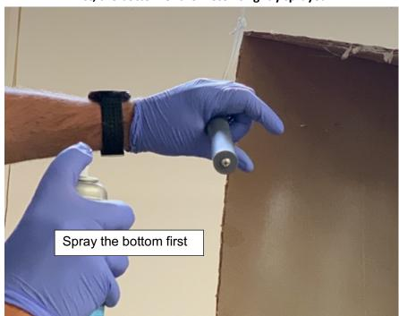
First, the bottom of the meter is lightly sprayed:
