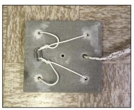
Figure 1A (top): Holes are drilled in the patio stone and each line is slipped through perpendicular holes. A loop is tied to end of each line. (Optional ground line is shown on right.)
