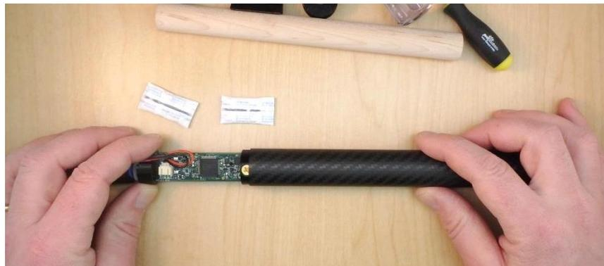
16. Add the two desiccant packs and push the circuit board and battery all the way into the housing. It may take a couple of attempts. Do not use excessive force.
