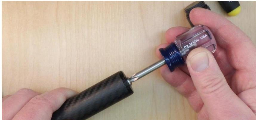
23. Flip back to the USB end of the housing and use the 3/32" hex driver to tighten the four hex screws taking turns to tighten them evenly by alternating screws. Once again, do not over torque.
