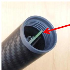
Check that circuit board overlaps with threads.
