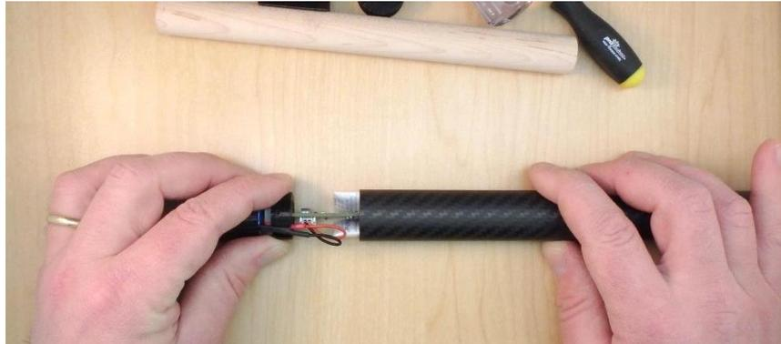
17. Temporarily install the nose cone. (The end cap will provide a stop for the circuit board assembly when inserted into the housing in the next step.)
